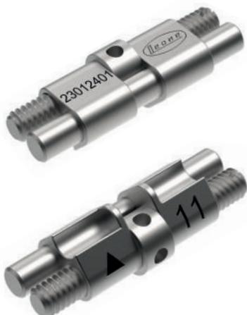
This expander is the optimized CAD-CAM version of the Stealth Easy Access. Instead of the arms, it has two transversal housings with an ending stop on the bodies that allow a perfect oriented coupling with the digitally designed and SLM manufactured framework, thus assuring an optimal laser welding process.
