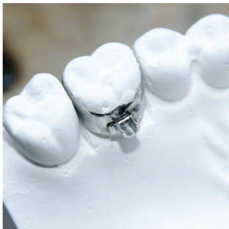
The connector's flanges ensure a good joint to the band by means of a welding machine
