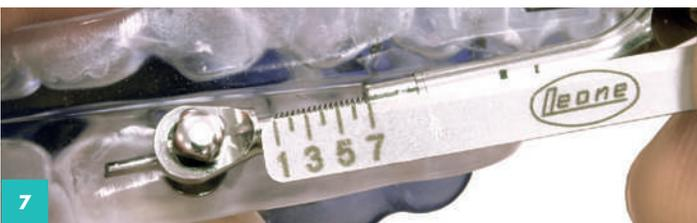
A ruler is laser etched on the wrench handle to check the activation length throughout treatment.
