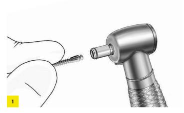
Once sterilised insert the head of the mini implant to the handpiece adapter Cat. 080-1002-00 (for Self-Drilling Orthodontic Mini implant) or Cat. 080-1002-01 (for Self- Drilling mini implants with closed dual slot) connected to a surgical micromotor.
