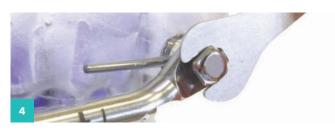
used in the laboratory to tighten the square head screws.
